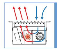
SoHo fan-powered linear terminals utilize crossflow fans to recirculate and condition air within an occupied space.
