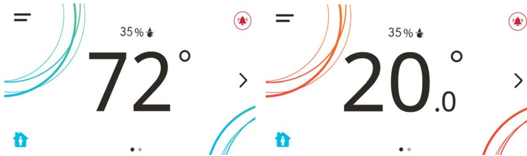
Figure 15: Thermostat controller home screen in cooling mode (left) and heating mode (right)
