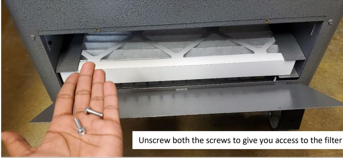
Unscrew both the screws to give you access to the filter and UV region
