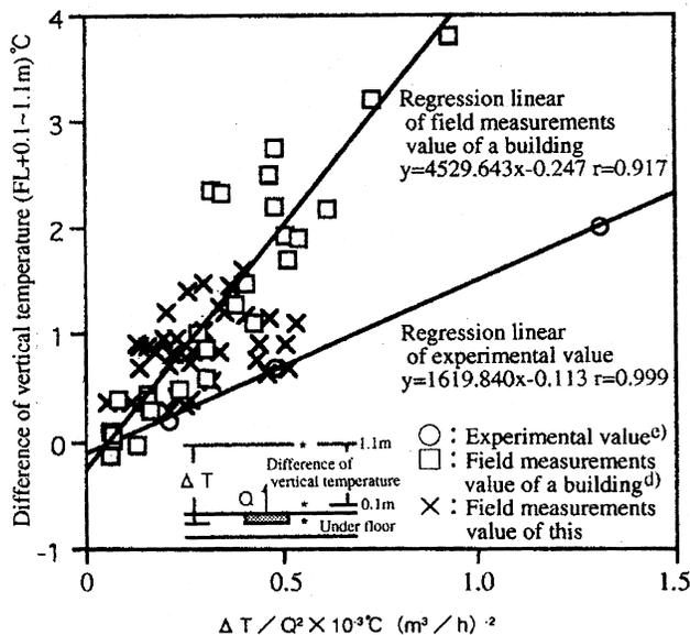
Figure 6 Relationship between  $\Delta T/Q^2$  and difference in vertical temperatures.
