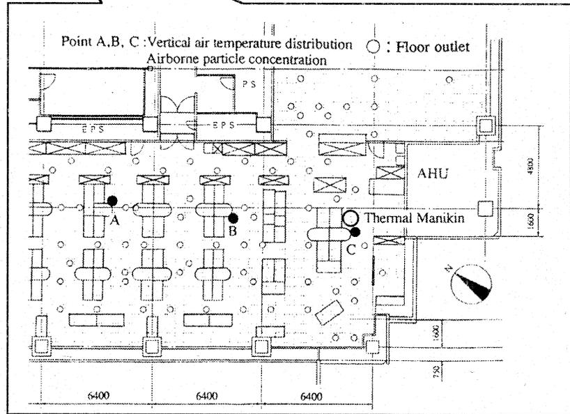
**Figure 2** Floor plan and measured areas with floor outlet layout (plan) on the underfloor air-conditioning floor and vertical temperature measurement points (\*AHU is air-handling unit).
