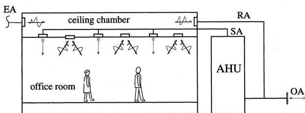
Overhead Air distribution (Ceiling-based) system
