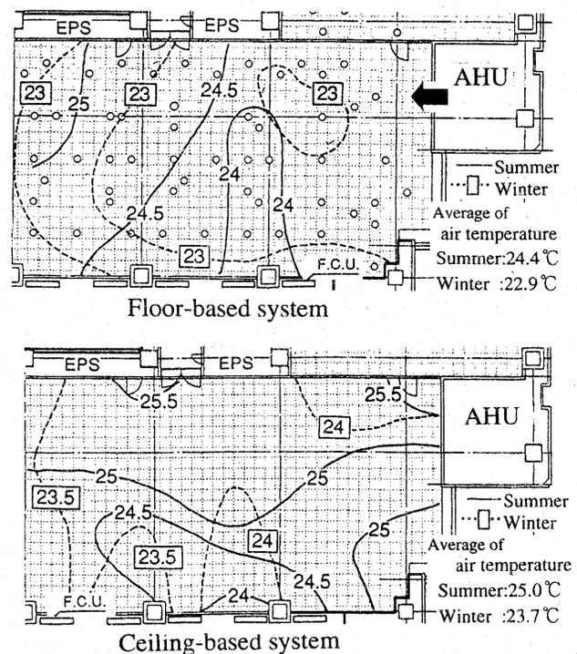
Figure 4 Horizontal distribution of air temperature at FL + 1.1 m.
