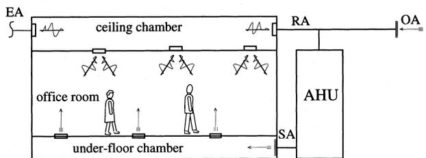
Underfloor Air Distribution (Floor-based) system
