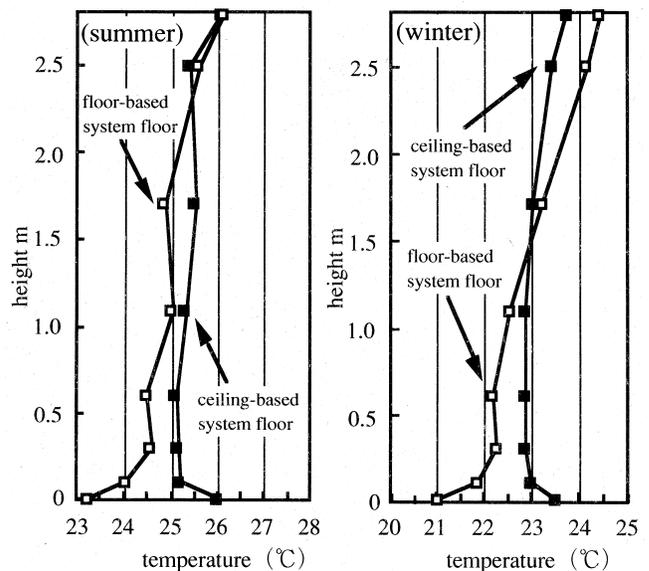
**Figure 5** Vertical air temperature distribution.
